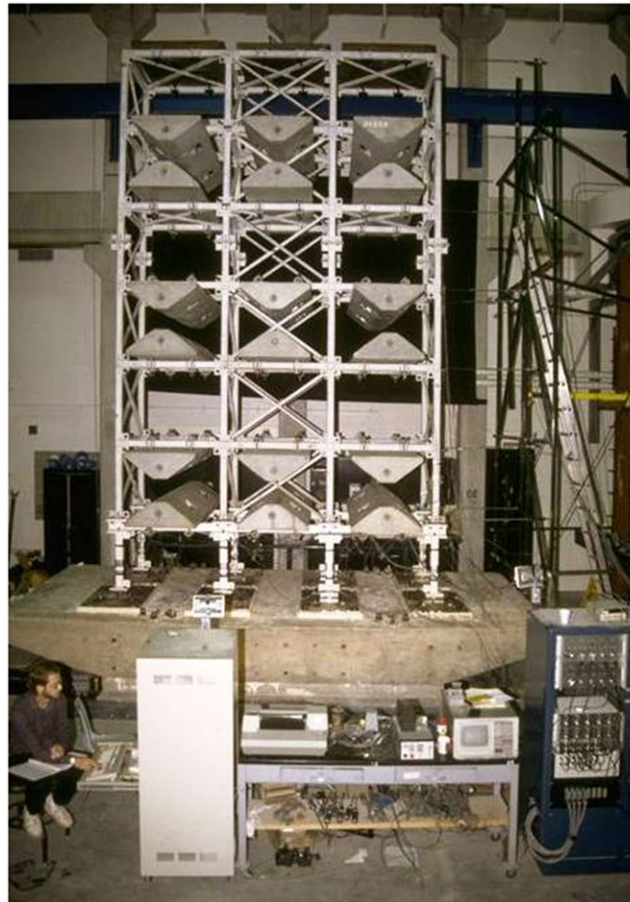
FIGURE 11 Seven-story model on the seismic simulator at the University at Buffalo, circa 1991. Courtesy of Michael C. Constantinou with permission [Colour figure can be viewed at wileyonlinelibrary.com ]
