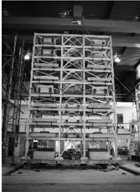
FIGURE 7 Nine-story, \frac{1}{4} scale model structure isolated on natural rubber bearings being tested on the shake table at the Earthquake Engineering Research Center of the University of California, Berkeley, in 1986. Courtesy of James M. Kelly with permission
