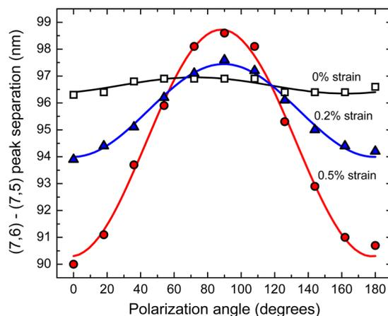
**Figure 4.** Polarization selectivity of differential spectral shift. The difference in peak emission wavelengths of (7,6) and (7,5) nanotubes in a polymeric coating is plotted against the angle between the axes of applied strain and excitation laser polarization. Applied strain magnitudes were 0 (open squares), 0.2% (triangles), and 0.5% (circles). The solid curves show best fits to the data using the function in eq 1.
