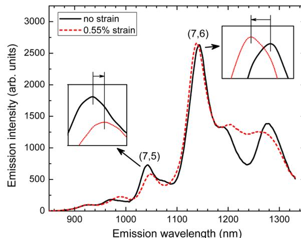
**Figure 2.** Changes in “strain paint” emission spectrum with applied strain. Emission spectra are shown for applied substrate strains of 0% (black solid line) and 0.55% (red dashed line). Insets illustrate the opposite shifts in peak positions for features dominated by (7,5) and (7,6) SWCNTs.
