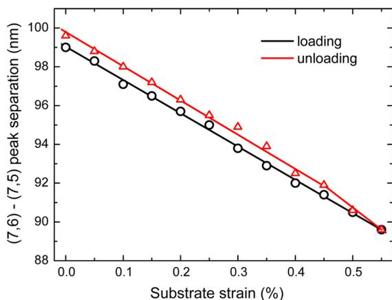
**Figure 3.** Strain variation of differential spectral shift. The difference in peak emission wavelengths of (7,6) and (7,5) nanotubes in a polymeric coating is plotted versus strain in the substrate, as measured with a resistive strain gage. Black circles show data measured with increasing strain; red triangles were measured with decreasing strain. Straight lines show linear best fits to the data.
