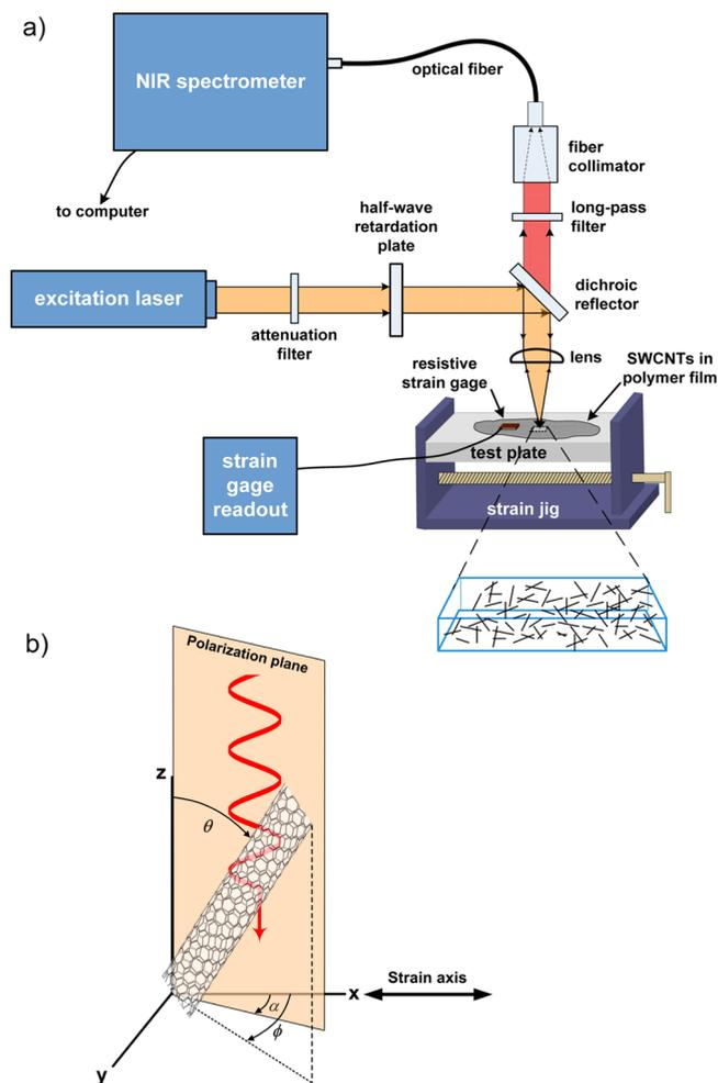
**Figure 1.** Schematic diagrams of (a) the experimental apparatus and (b) angle definitions.
