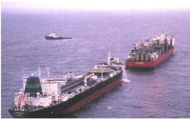
Fig. 1 Offloading of a FPSO by shuttle tanker and tugs
