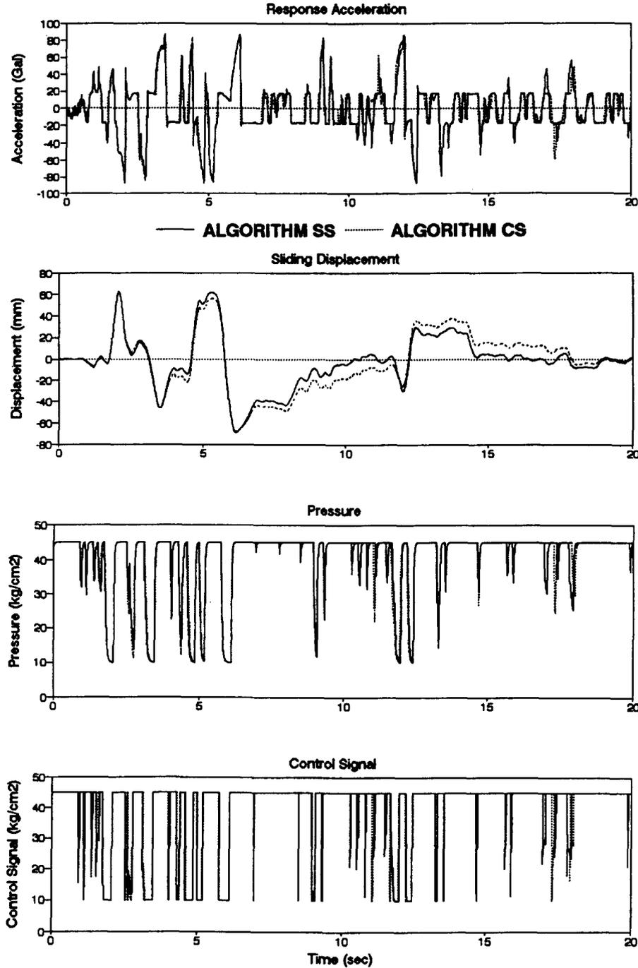
Fig. 5. Comparison of simulated responses, using algorithm SS and algorithm CS, under 1940 NS El Centro earthquake input (300 Gal).
