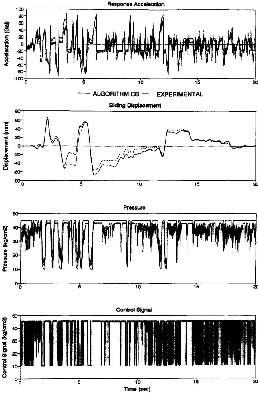
Fig. 4. Comparison of measured and simulated responses, using algorithm CS, under 1940 NS El Centro earthquake input (300 Gal).
