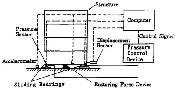
Fig. 1. Friction controllable sliding isolation system for buildings.
