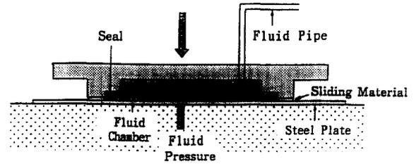
Fig. 2. Idealized view of friction controllable bearing.
