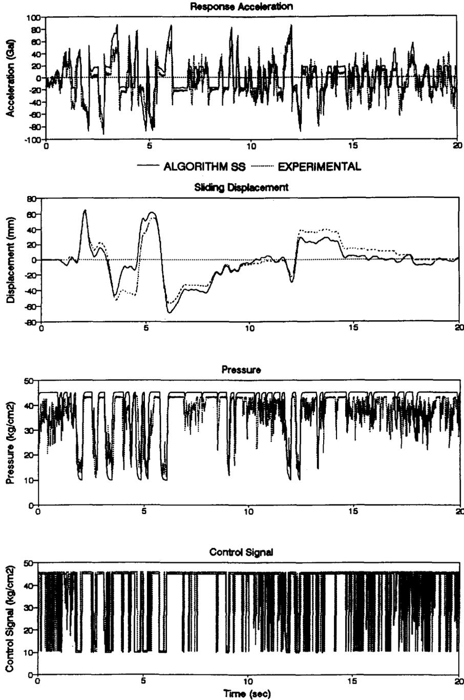
Fig. 3. Comparison of measured and simulated responses, using algorithm SS, under 1940 NS El Centro earthquake input (300 Gal). The responses shown are: response acceleration of the rigid structure; sliding displacement of the rigid structure; pressure in the bearing fluid chamber; and pressure control signal from the computer. 1 Gal = 1 cm/s<sup>2</sup>.
