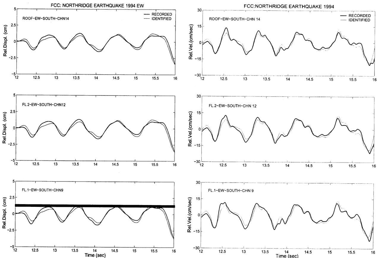
Fig. 6. Comparison of recorded and simulated time history response obtained from 12 to 16 s. Time segment identification (a) displacement response (thick line shows the gap for one sided impact); (b) velocity response.
