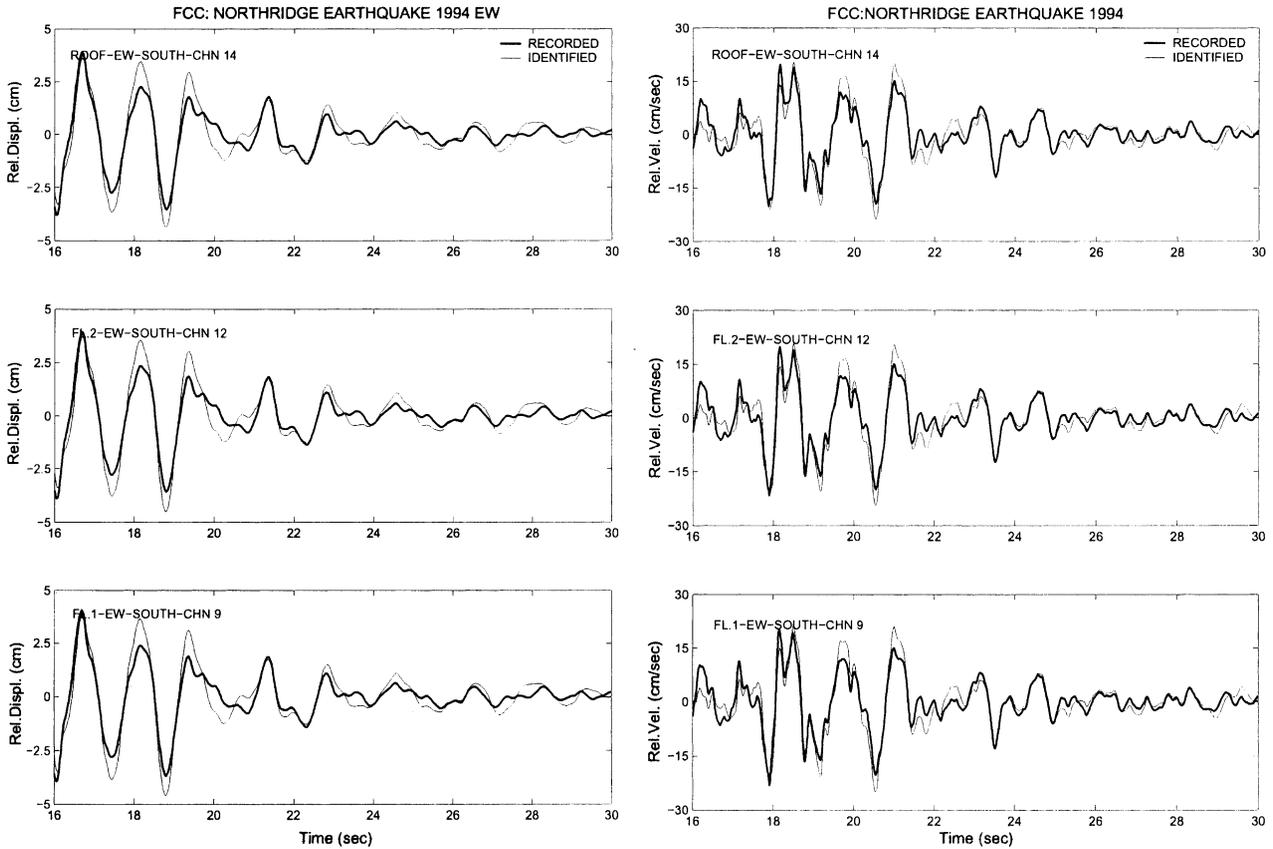
Fig. 7. Comparison of recorded and simulated time history response obtained from 16 to 30 s time segment identification (a) displacement response; (b) velocity response.
