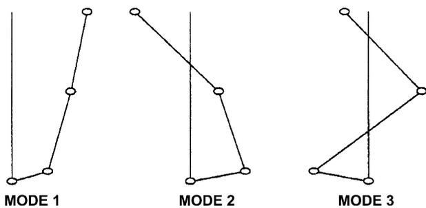
Fig. 8. Modal response in EW direction during impact.
