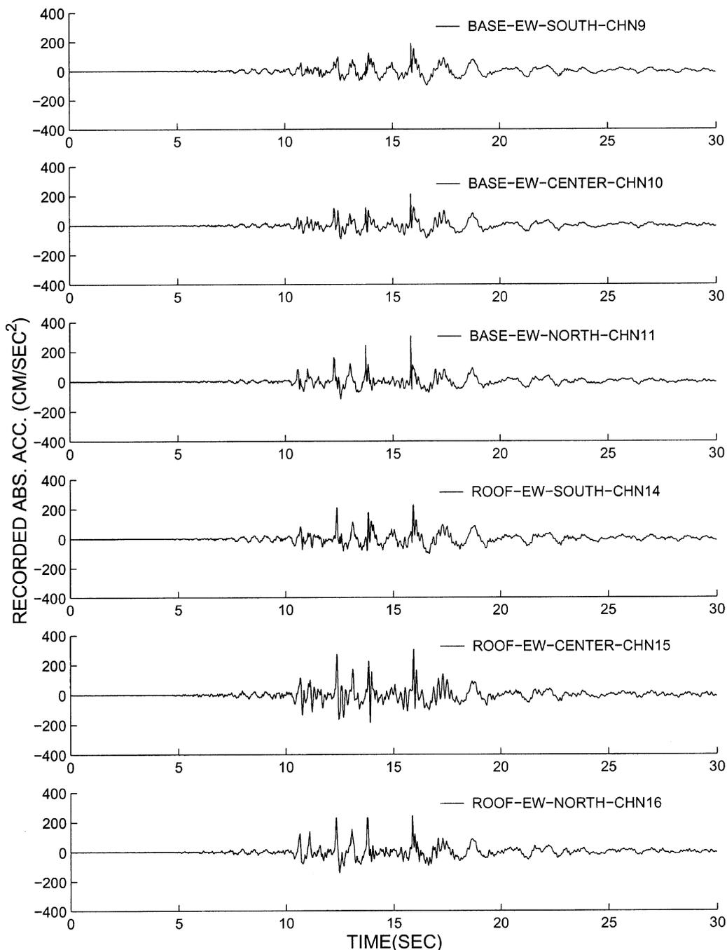
Fig. 3. Recorded acceleration time histories of FCC building in Northridge earthquake.
