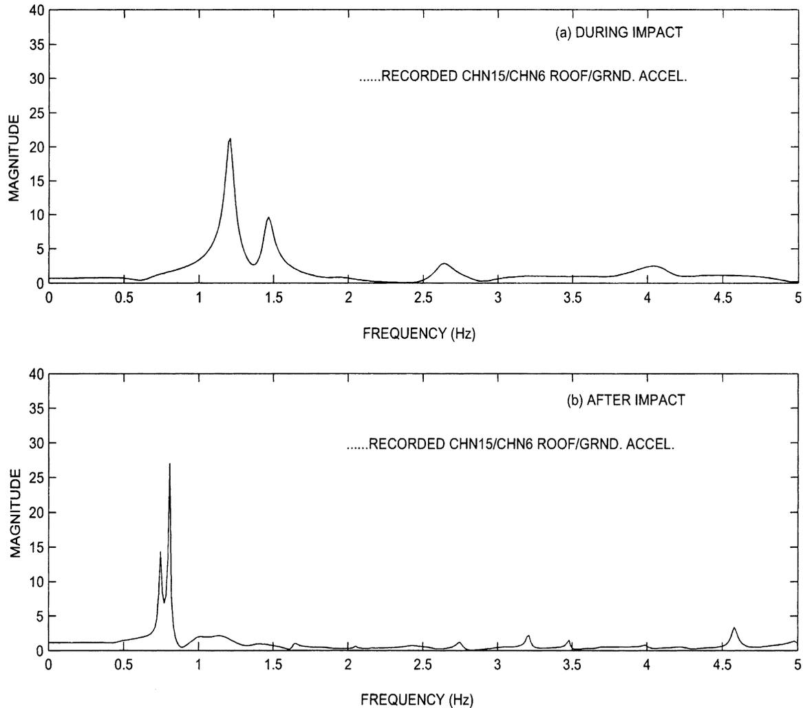
Fig. 10. Recorded transfer function in EW direction: (a) base isolation with impact; (b) base isolation without impact.
