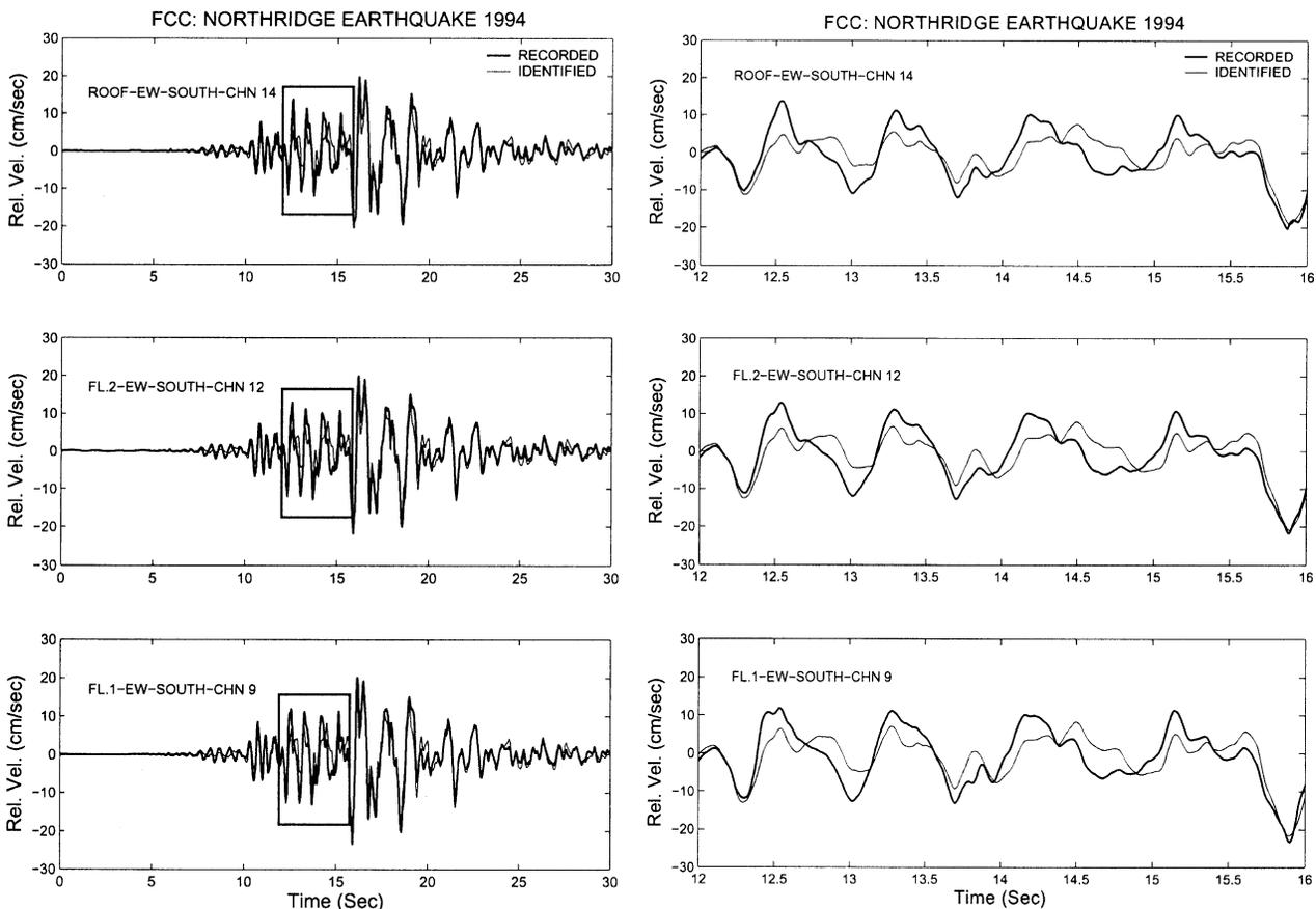
Fig. 5. Comparison of recorded and simulated velocity response obtained from 0 to 30 s identification (a) time history response from 0 to 30 s; (b) 12–16 s response time history magnified to show the differences in identified and recorded responses.
