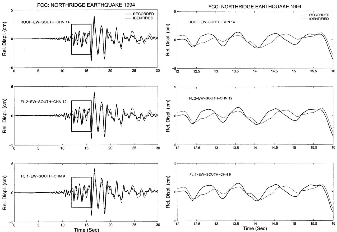
Fig. 4. Comparison of recorded and simulated displacement response obtained from 0 to 30 s Identification (a) time history response from 0 to 30 s; (b) 12–16 s response time history magnified to show the differences in identified and recorded responses.
