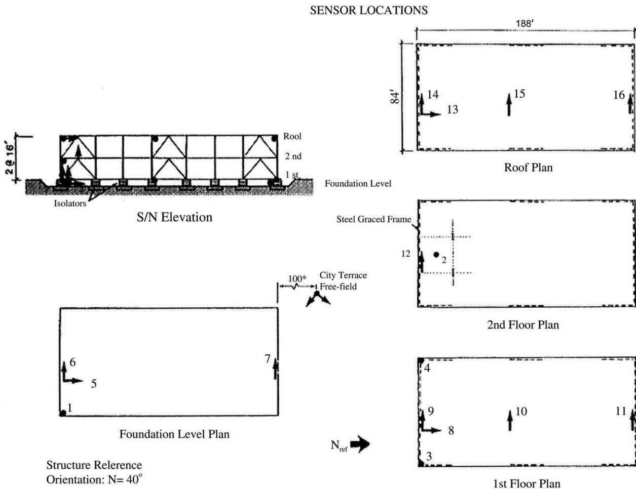
Fig. 2. FCC building elevation and sensor locations.
