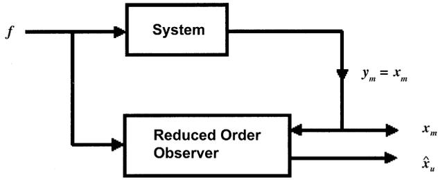
Fig. 1. Block diagram showing reduced order observer.
